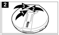
While the PROG indicator is blinking, select the desired preset using the PRESET  $\blacktriangle$  ① or  $\blacktriangledown$  ② button, then press the PROG button ③ to set the memory.
